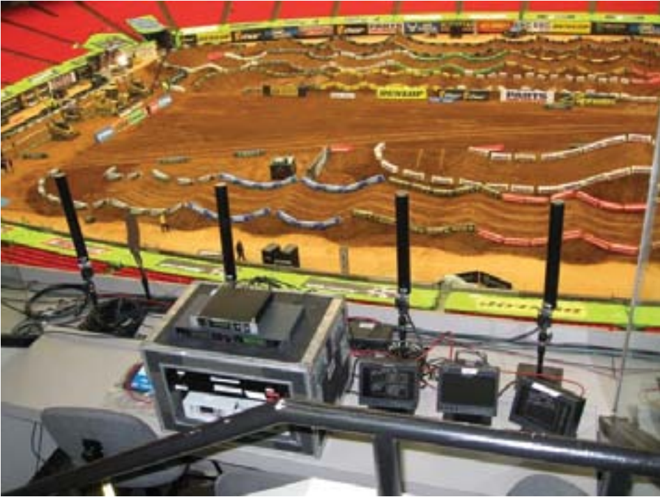
Four SCR225-12 compact sector antennas in a diversity receive set-up inside stadium.
