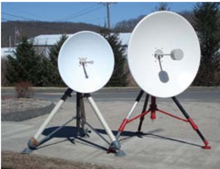
Reflectors R1 and R3, with in-line 6 GHz band feed and 1.5 GHz feed, respectively.
