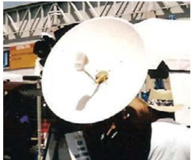
Reflector R1 with 6 GHz band feed R1Feed675 in use tracking helicopter transmissions.
