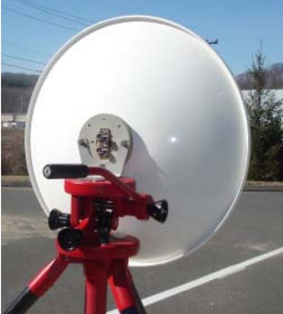
Rear view of ReflectorR1 with dual-polar feed (right).
