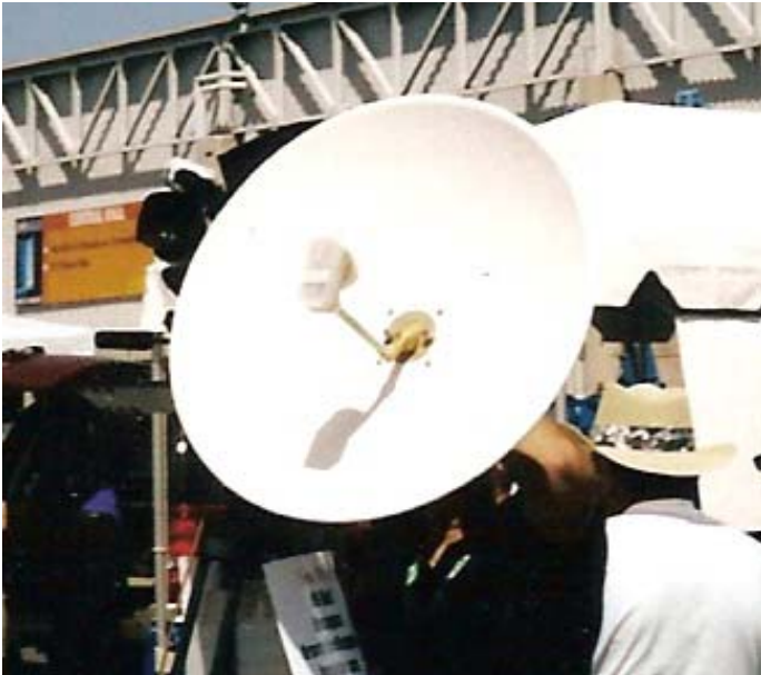
ReflectorR1 with 6GHz band feed R1Feed675 in use tracking a helicopter transmission (above).
