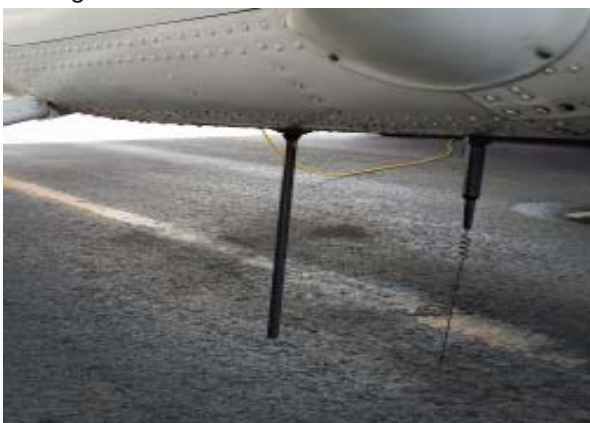
Below: 2GHz omni on Cessna fuselage.
