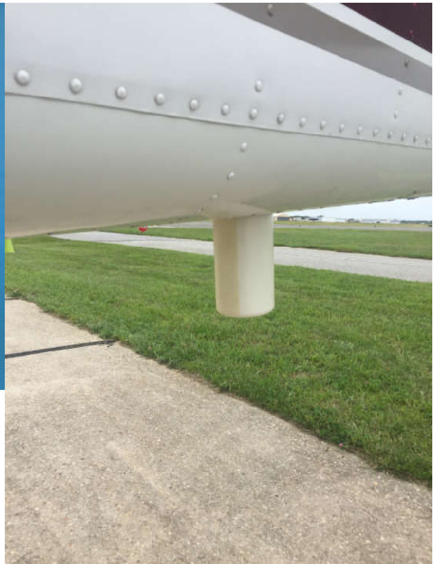
WHO225 antenna mounted on light aircraft (right).
