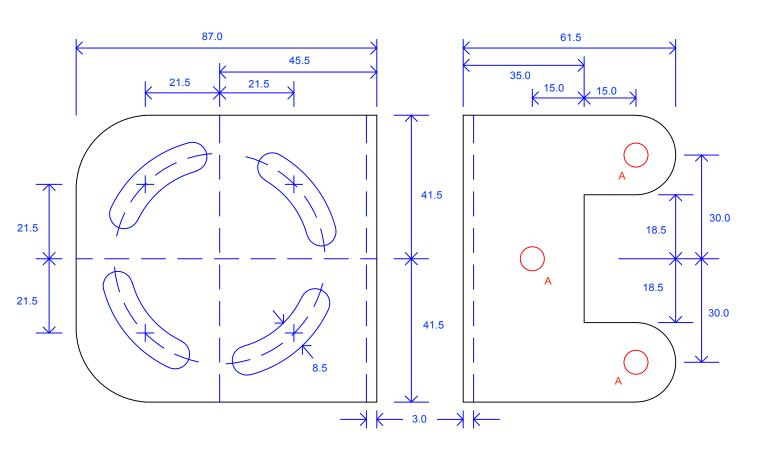
Note: Slots allow -20° to +30° tilt. Use with U-bolt size 5/16" - 18, 1 3/8" inside arms (McMaster-Carr part no. 8896T69).
